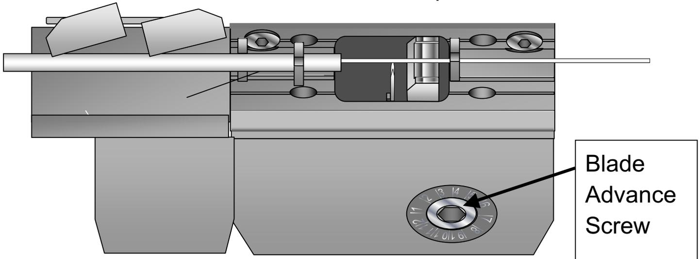
Using the hexagonal screwdriver supplied, turn the blade adjustment screw clockwise by  $30^\circ$  so the indicator mark is aligned opposite the next mark on the circular scale
