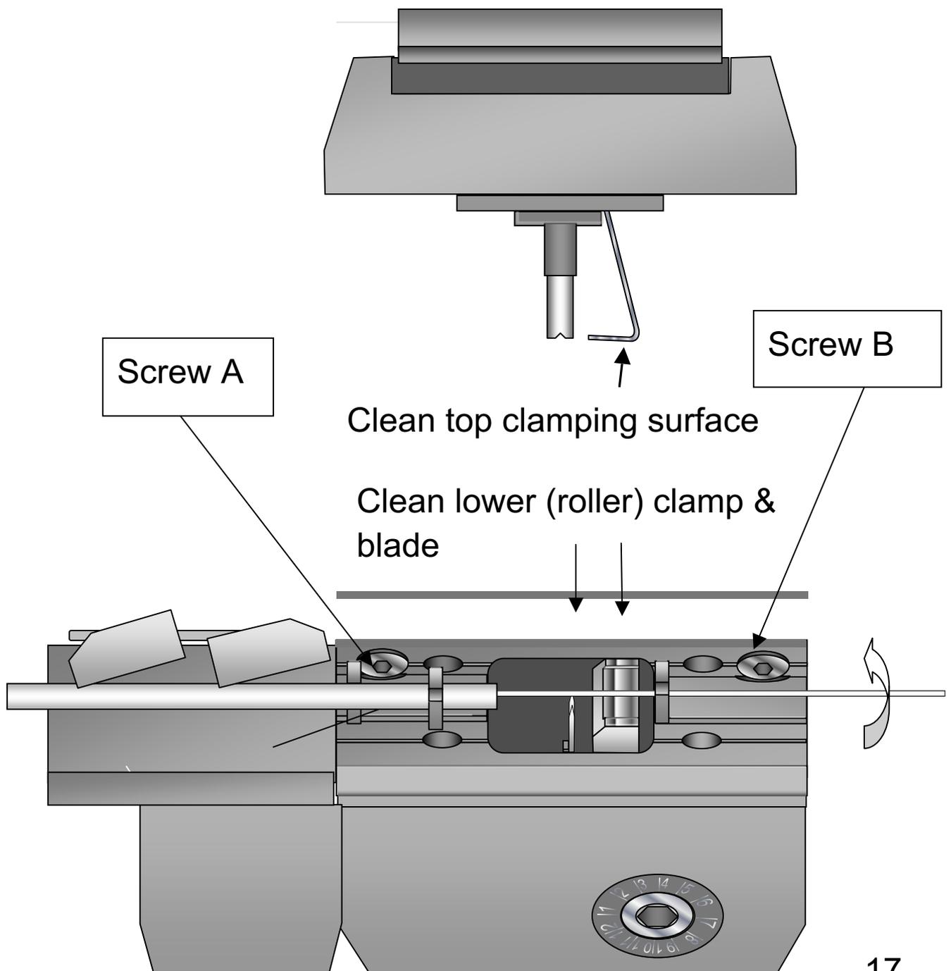
The lower clamps should be cleaned with an alcohol wipe, rubber, wood or other non-hard material. Do not touch the diamond blade.
