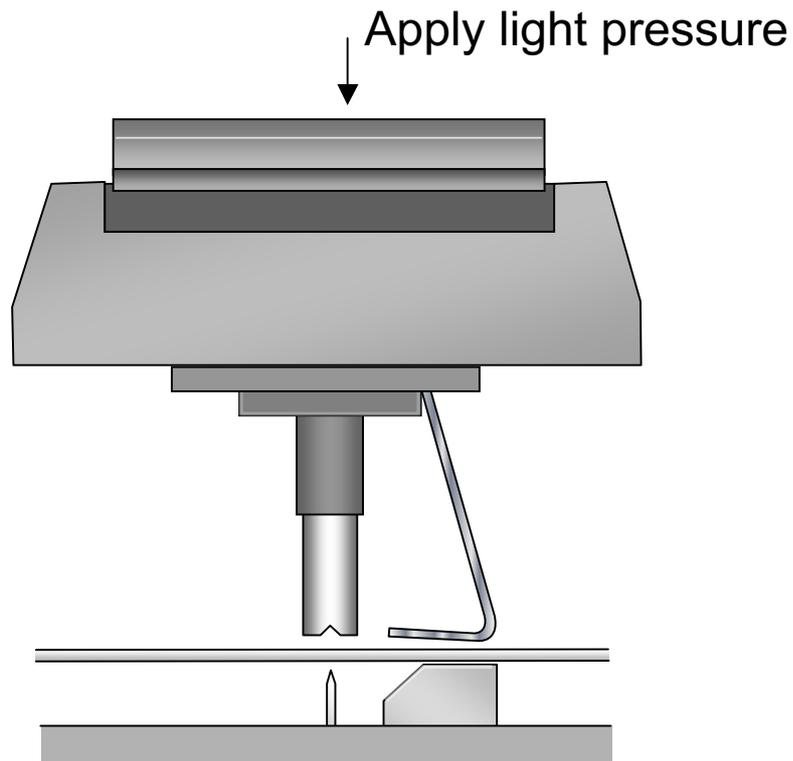
Release the pressure on the cleaver top handle as soon as the fiber cleaves.
